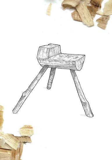
"Biting interferes with the state of flow required for efficient axing. This is eliminated with an across grain block.
